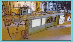
1" Bema Model G1AD Hydraulic Tube Bender
