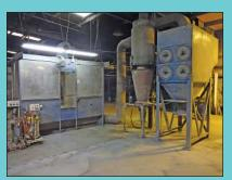
36" Wide X 10' Long X 9' High Manual Steel Pass Thru Single Station Powder Coat Spray
