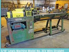
5/16" Lewis Machine Model No. 2CV Wire Straight
