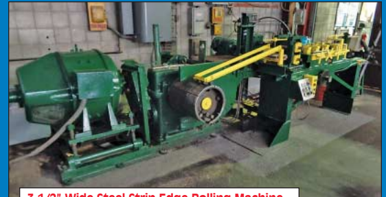
3-1/2" Wide Steel Strip Edge Rolling Machine
