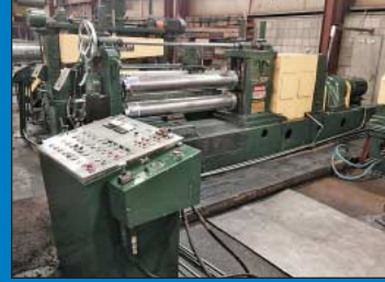
52" Wide x .250" Thickness X 40,000 Lb. Paxson Slitting Line
