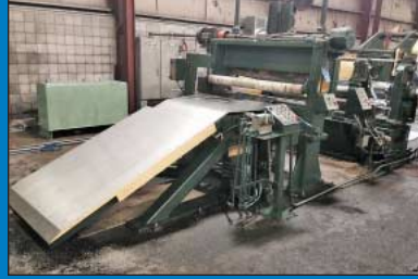
52" Wide x .250" Thickness X 40,000 Lb. Paxson Slitting Line
