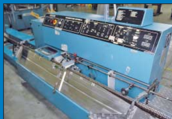
Sheridan "Pacesetter" Model SP705A Eight-Pocket Saddle Stitching System
