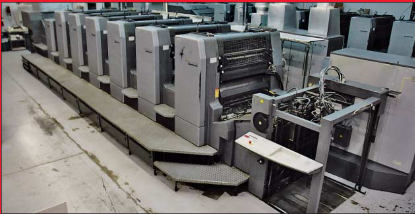
Heidelberg Model Speedmaster SM102-8-P5-S Eight-Color Sheet Feed Offset Perfecting Printing Press
