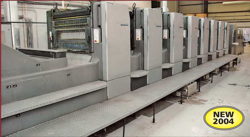
Heidelberg Model Speedmaster SM102-8-P5-S Eight-Color Sheet Feed Offset Perfecting Printing Press
