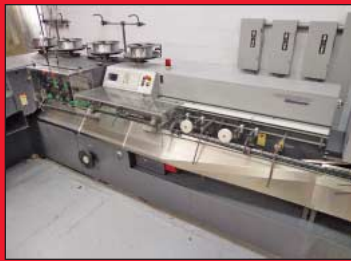
Heidelberg Model Stitch 270A Master Six-Pocket Saddle Stitching Line
