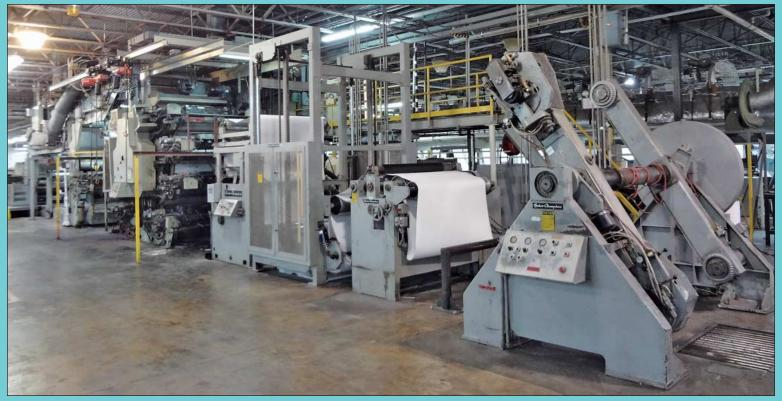
55" Wide Kidder-Stacey Model 660Z Centraflex / Bobst Champlain Lemanic S1425 8-Color Roll to Sheet Central Impression Flexographic Printing Press Line
