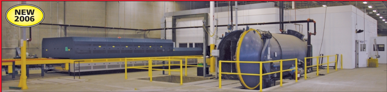
Overall View Tamglass Model ProL-2000-2636 Flat Glass Laminating Line With Tamglass Eurotherm Autoclave
