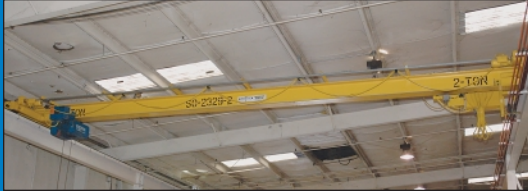
2 Ton X 30' Approx. Span X 75' Approx. Long Progressive Crane Inc. Free Standing Overhead Bridge Crane System
