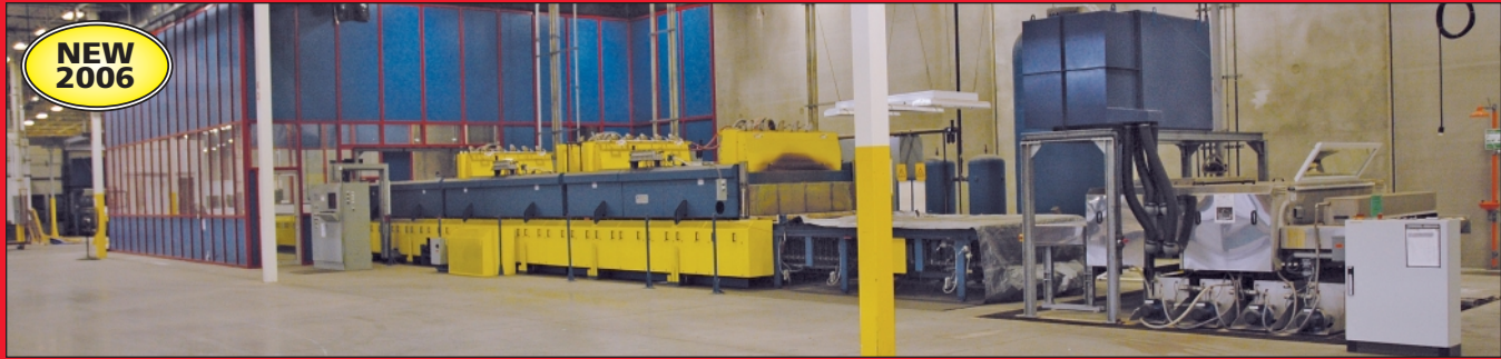
Overall View Tamglass Model CBHF 72" X 144" - 3Z-2Q-PT3.0 Flat Glass Horizontal Continuous Tempering Furnace
