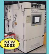
Cincinnati Sub-Zero Model ZH-32-305-SCT/ **Environmental Test Chamber**
