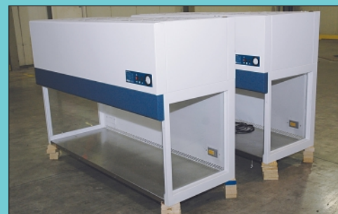
(2) 5' Esco Laminar Flow Cabinets
