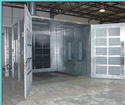
12' W X 14' L X 10' High Binks Modular Galvanized Panel Rear Draft Spray Booth
