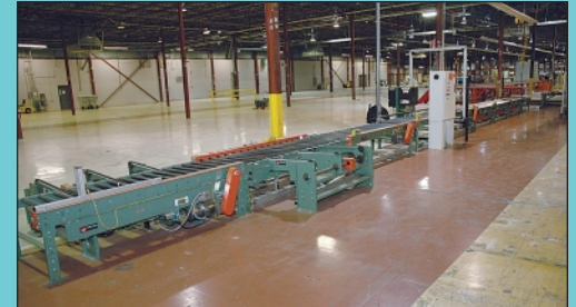
30' Wide X 80' Long Roach Motorized Conveyor Strapping Line
