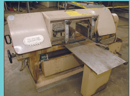
13" X 20" Kalamazoo Model 13AW Horizontal Band Saw
