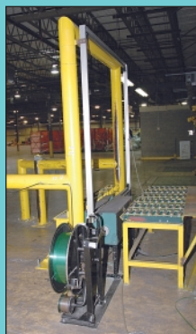
(2) 6' X 6' Signode Model MCD 500 Automatic Strappers
