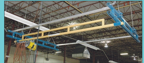
(2) 500 Lb. Gorbel Ceiling Hung Rail Systems w/ 200 Lb. & 320 Lb. Zimmerman Balance Air Tool Balancers
