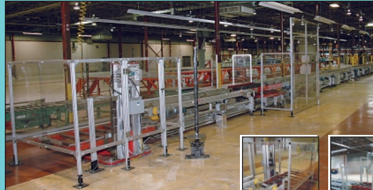
40' Wide X 200' Long Tekno Gemini 25-Station Hot Rail Modular Aluminum Assembly Conveyor
