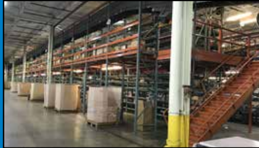
INTERLAKE 250' x 50' x 208" T Pick-to-light Module
