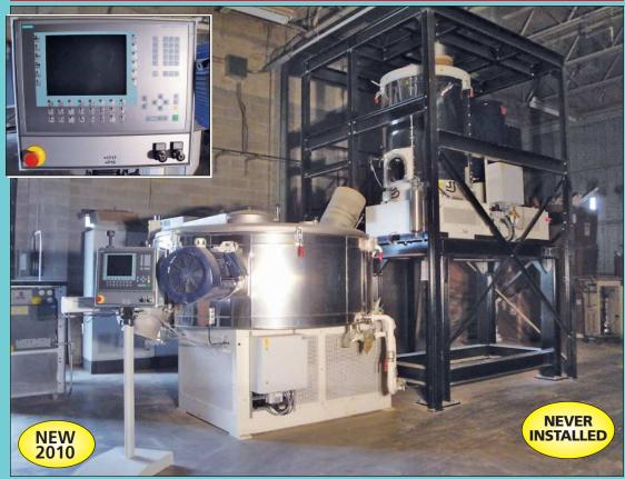
\*\*1,200 Liter MTI Model M1200 High Intensity Heating Mixer and \*\*3,060 Liter MTI Model KMV-3000 Cooler
