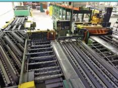
60" Engel Model 5-16 Square Duct Fabricating Line with TDF Duplex Rollformer
