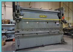
12' Cincinnati Series 90-10 Mechanical Power Press Brake
