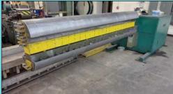
10' Ovalformer Model OF-1018 Spiral Duct Tube Ovalizer
