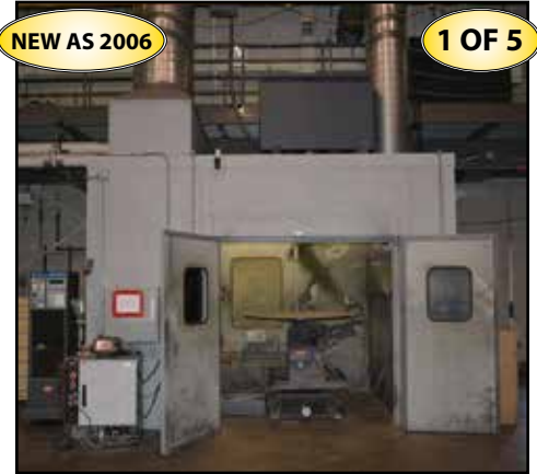
(5) SULZER METCO & HOBART TAFA Thermal Spray Metallizing Systems
