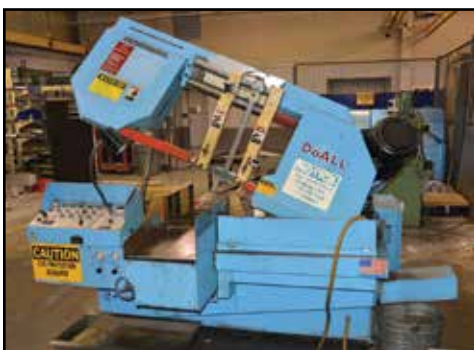
DOALL 16" x 16" Horizontal Band Saw
