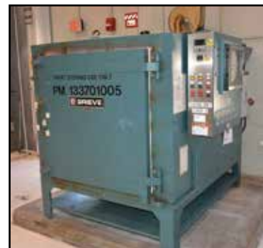
GRIEVE 1,050° Single Door Batch Oven
