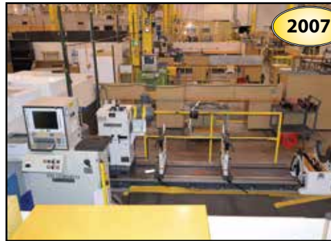
2007 SCHENCK HML5U Horizontal Balancer
