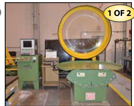
(2) SCHENCK VE40L Vertical Balancers
