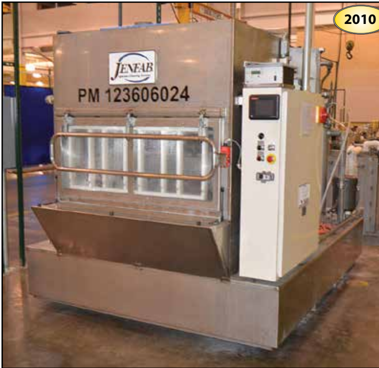
2010 JENFAB Lean Clean S.S. Aqueous Basket Type Parts Washer
