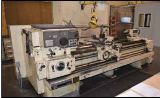
(2) LODGE & SHIPLEY 20" x 80" Engine Lathes
