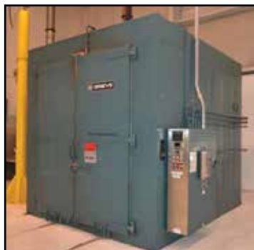
GRIEVE 1,050° Walk-In Electric Furnace
