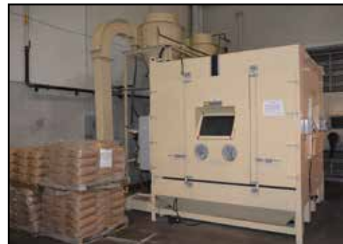
ABRASIVE BLAST SYSTEMS 8' x 8' x 6'H Blast Booth
