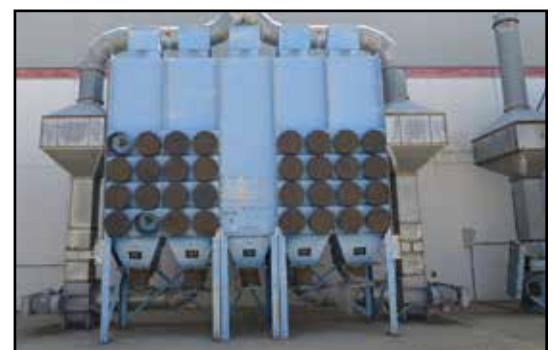
TORIT DFT4-64 Dust Collector
