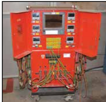
COOPERHEAT 6-Way Power Source Control Console
