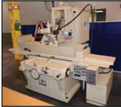
GALLMEYER & LIVINGSTON 16" x 36" Surface Grinder
