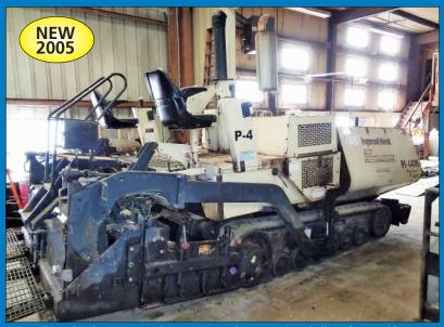
Ingersoll Rand / Blaw Knox Model PF-4410 Track Mounted Asphalt Paving Machine
