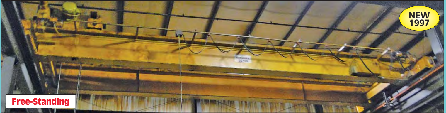
25 Ton X 35' Approx. Span X 125' Approx. Long Crane Builders Inc. Free Standing Double Girder Top Running Overhead Crane System
