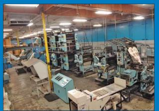
22.75" X 35" Wide 22-Color Tensor Web Coldset Press Line Consisting Of (4) Tensor T1400 Four-High Print Towers w/ Tensor H50 Folder & Goss SC Folder
