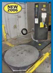
60" Wulftec Model WSML-150-B Rotary Stretch Wrapper
