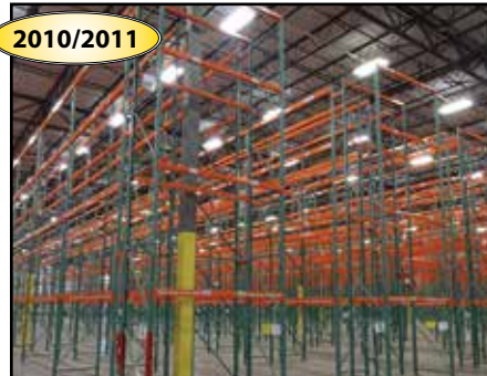
(66) Sections ESP F20 42"D X 24'H X 90"W Teardrop Adjustable Beam Pallet Racking
