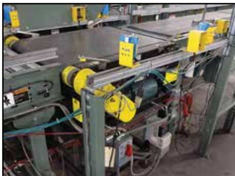
(2) METTLER TOLEDO IND9D56 Rubber Belt Conveyor Scales
