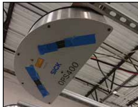
(5) SICK OPS400 Digital Bar Code Scanners
