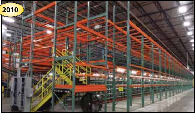
(2) 2010 ESP Two-Level Pick Modules, Approx. Dimensions 50'W X 300'L x 18'T
