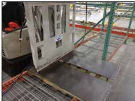
CASCADE R35F-QPB-0001 3,500-lb. Push / Pull Attachment
