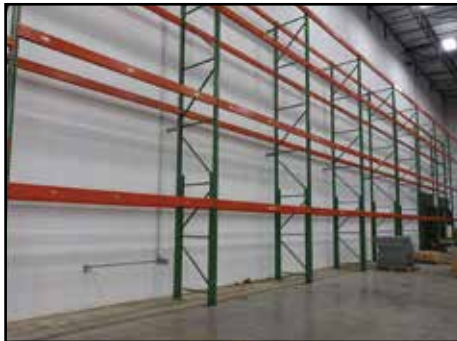
(8) Sections INVINCIBLE IV48 42"D X 24'H X 12'W Teardrop Adjustable Beam Pallet Racking
