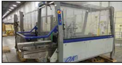
O/K DURABLE PACKAGING Superformer 1 Case Erector
