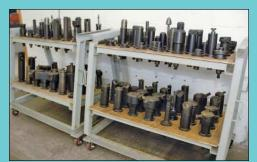
(195) No. 50 and Taper and (78) No. 40 Taper Tool Holders
