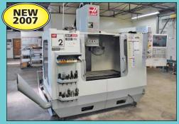
Haas Model VF-2D/YT CNC Vertical Machining Center
