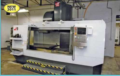
Haas Model VF-9/50 CNC Vertical Machining Center
