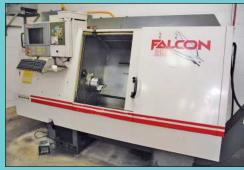
Cincinnati Milacron Model Falcon 200 ERL Slant Bed Two-Axis CNC Turning Center
