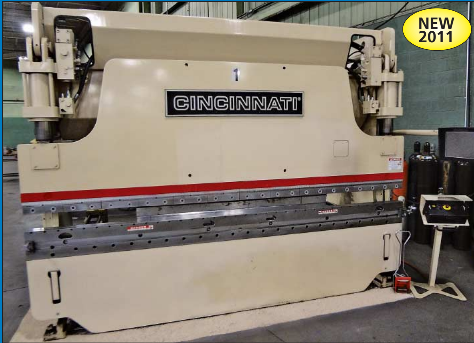
90 Ton x 12' Cincinnati Model 90PFX10F Proform CNC Hydraulic Press Brake
