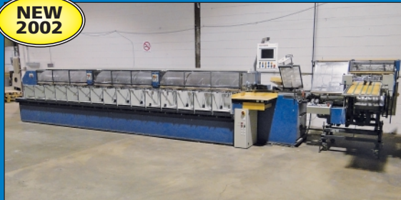
Theisen & Bonitz Model TB Flex B315VP 15-Pocket Collator
