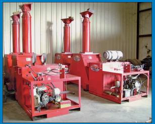
400 Ton Lift Systems Model 44A Four-Point LP Gas Hydraulic **Gantry System**
