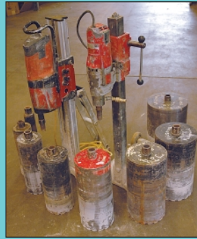
Partial View Core Drilling Machines and Diamond Bits
