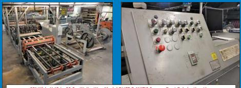
60" Wide X 18 to 26 Ga. Welty-Way Model DUCT-O-MATIC Square Duct Fabrication Line
