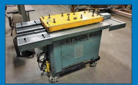
20 Ga. Engel Model M-800-S S-Drive & Snap Lock Rollformer
