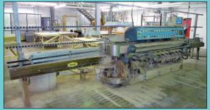
Bovone Electromeccanica Model Mini-Max 371 Pass-Thru Vertical Edge Glass Beveler
