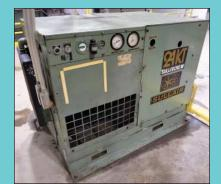
40 HP Sullair Model 10-40L Cabinet Enclosed Rotary Screw Air Compressor
