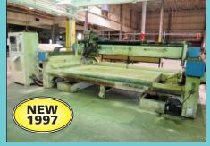
69" X 118" Intermac Model Master Groove 1500 Three-Axis Gantry Type CNC Glass Grooving
