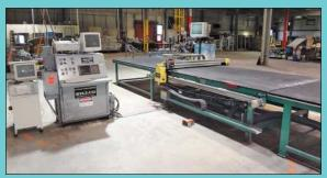
78" X 120" Billco Two-Axis Bridge Type CNC Glass Cutting Table
