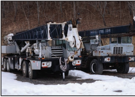
FWD/GROVE 18-TON & GROVE 35-TON TRUCK CRANES
