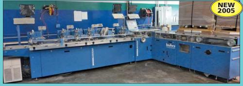
Buhrs Model BB300-10K Six-Station Automatic Inserting System
