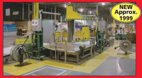
Signode Model MOD-710 Dual Strapper Semi-Automatic Strapping & Transfer System
