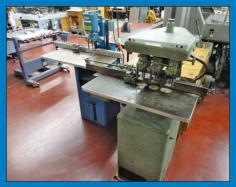
Three-Spindle and Single-Spindle Paper Drills
