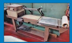
14" X 20" Clamco "L" Heat Sealer / Shrink Tunnel
