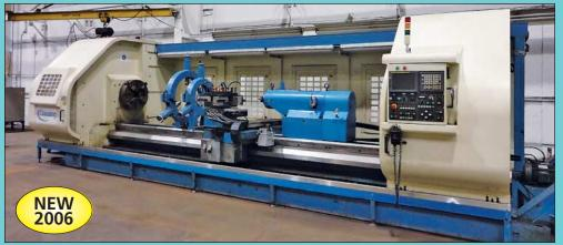
42" x 192" Clausing Model CL45200 Flat Bed CNC Lathe
