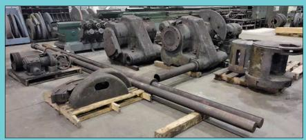
(2) Pot Chuck Heads for Cranks Shafts
