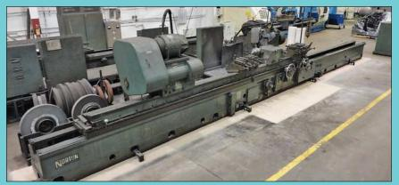
24" x 192" Norton Combination Crankshaft and O.D. Cylindrical Grinder
