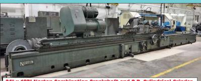
x 192" Norton Combination Crankshaft and O.D. Cylindrical Grinder
