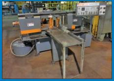
12" x 12" Hem-Saw Model H90A-4 Automatic Horizontal Band Saw
