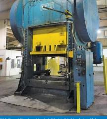
700 Ton Minster Model 50-11-84 Straight Side **Double Crank Press**
