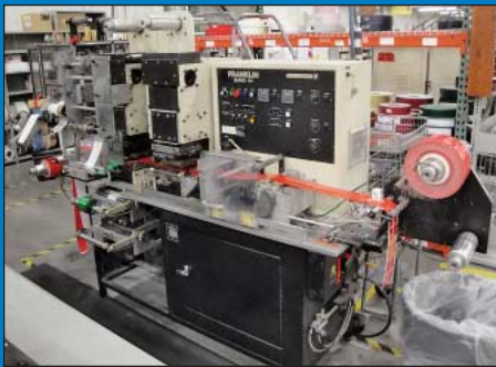
(2) Franklin Model 164 Generation II Roll to Roll Hot Stamp & Die Cut Label Press
