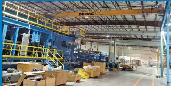
**3 Ton x 60' Approx. Span x 90' Approx. Long Demag Free-Standing Overhead Bridge Crane System
