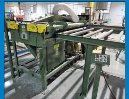
72" Lauderdale-Hamilton 50-HP Rip Saw w/ In-Feed and Out-Feed
