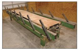
Ruvo Model 2210 Pneumatic Staircase Assembly Clamp
