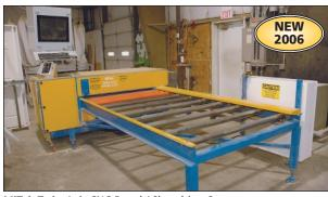
MiTek Twin-Axis CNC Panel / Sheathing Saw
