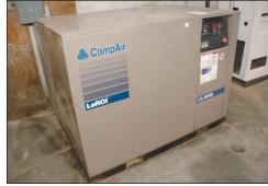
40 HP LeRoi Model Compair CL40SS Cabinet Type Rotary Screw Air Compressor
