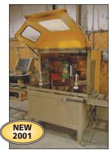
Merrick Triad Model SSR Smart Stair CNC Stair Router
