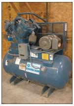
25 HP Quincy Model QR5120EST Two-Stage Horizontal Tank Rotary Screw Air Compressor
