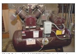
15 HP Quincy Model 2153D12HCA Horizontal Tank Two-Stage Air Compressor
