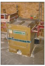
14" Powermatic Model MMM Upacting Cut-Off Saw
