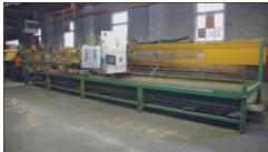
(2) Mitek Model 7000000/4000 CNC Truss Saws
