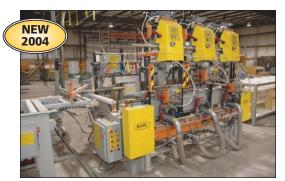
BAMC Builders Automation Machinery Co. Model 625/1550 REM Automatic Pre-Hung Door Machine
