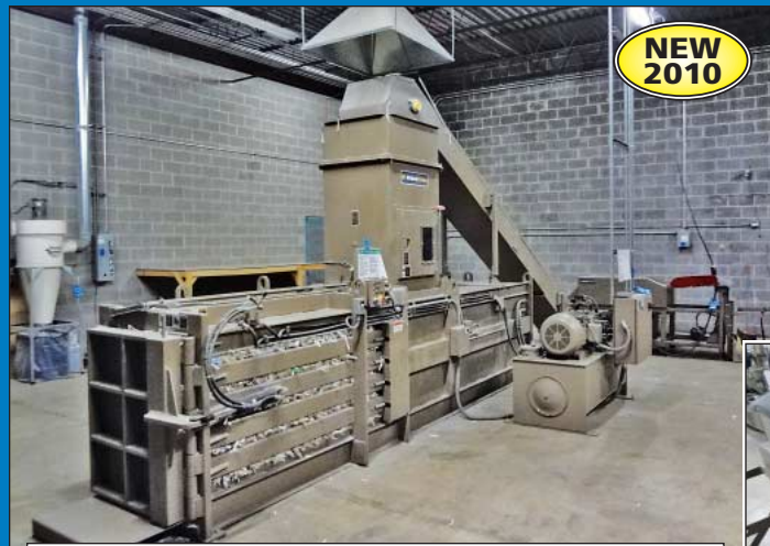
Allegheny Model 3430-2572CE Closed End Horizontal Hydraulic Baler, Allegheny Model Model 16-150C Shredder, Incline Conveyor, & Tipper – Madison, Ohio Location
