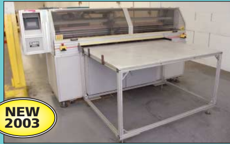
60" T-ROC Equipment Model ABM60-3H Programmable Custom Box Maker
