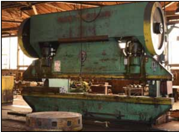
CLEVELAND CRANE 400-Ton x 18' Mechanical Press Brake
