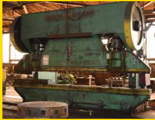
(2) CLEVELAND CRANE 400-Ton Mechanical Press Brakes
