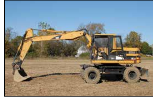
CATERPILLAR M312 Wheel Excavator
