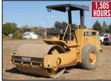
CATERPILLAR CS-433C 66" Single Smooth Drum Compactor
