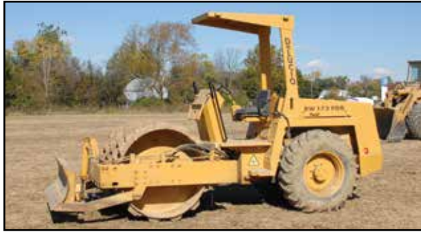
BOMAG BW172PD 66" Single Sheep's Foot Drum Compactor
