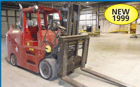
30,000 LB Taylor Model TC-300 Solid Tire LP Gas Lift Truck
