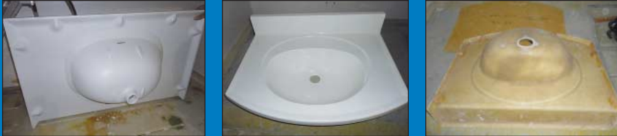
(18) Various Molds to Produce Various Size Vanity Tops, Overflows & Sample Plaque Molds
