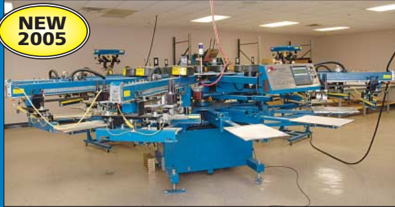
20" X 28" Progressive Model Falcon EF1012E 10-Color 12-Station T-Shirt Press
