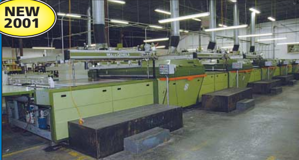
60" X 70" Sias Multiforma Five-Color In-Line Press (UV) w/ Automatic Sheet Stacker
