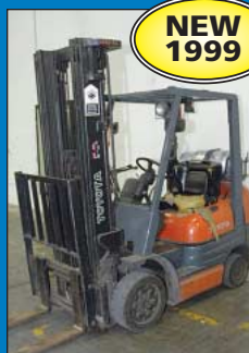
5,000 Lb Toyota Model 42-6FGCU25 LP Gas Solid Tire Lift Truck
