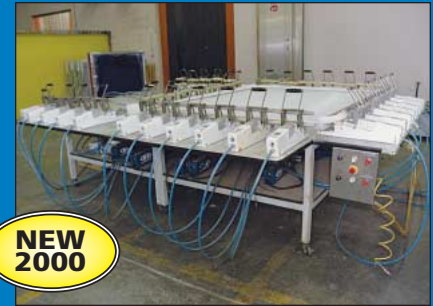
73.5" X 114.5" Saati Pneumatic Power Ten-Clamp Screen Stretching System
