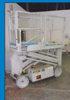
Strato Model FRX-16 Self Traveling Electric Scissor Lift Platform
