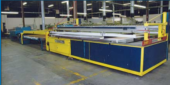
62" X 144" American Long Stroke Flat Bed Screen Printing Press
