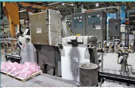
Ajax Magnethermic Model 150-A Two-Station Induction Melting Furnace
