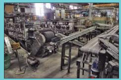
Spang Type K-5178 3-Zone Electric Belt Type Annealing Furnace
