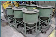
(25) 48" Diameter x 45" Tall Cone Type Bottom Dump Hoppers
