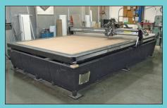
Cybermation Autograph Multi Cutter 8000 Three-Axis CNC Sign Router
