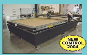
Multi-Cam Cybermation Autograph Multi-Cutter 8000 Two-Axis CNC Sign Router
