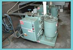
(2) 25 HP Gardner Denver Model EBEQFB Electric Saver II Skid Mount Air Compressors
