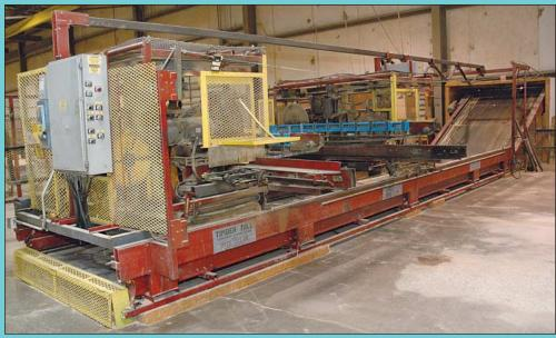
imber Mill Model 6-20E Six-Blade Component Saw
