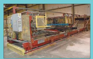
Timber Mill Model 6-20E Six-Blade Component Saw
