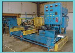
Clary Master Model 329 Four-Blade Component Saw
