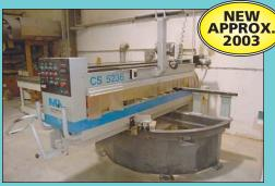
Midwest Automation Model CS5236-16 Cutting Station Postforming Saw
