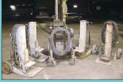
(4) 12 Ton Hydraulic House Jacks w/ 7-1/2 HP Electric Hydraulic Power Unit
