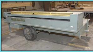
Glass Master Model 215-3BT Grooy-Master Duct Board Machine
