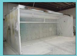
21'W X 8'D X 11'H Mfg. Unknown Bolt Together Rear Exhaust Calvanized Steel Paint Booth
