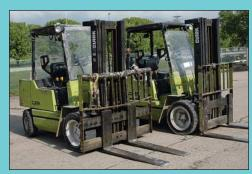
Partial View (2 of 5) Clark Solid Pneumatic Tire Lift Trucks To 6,500 Lb. Capacity
