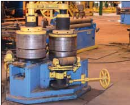
4" x 4" x 1/2" Approx. Capacity JPT Built Mechanical Power Vertical Angle Bending Rolls
