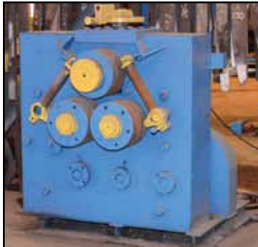
3" x 3" x 3/8" Approx. Capacity JPT Built Mechanical Power Horizontal Angle Bending Rolls
