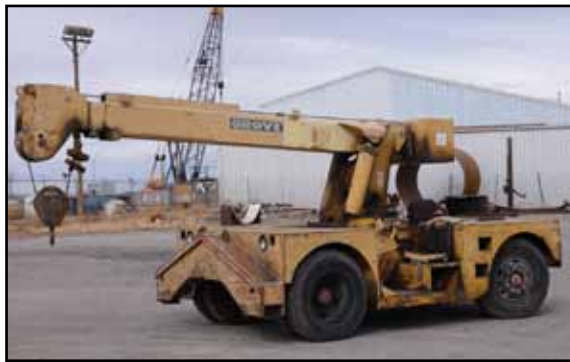
GROVE 12,000-lb. Carry Deck Crane
