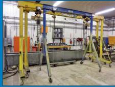
(2) 2 Ton x 16' Span Contrx Model GL-16 Portable A-Frame Gantry Cranes
