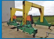
(2) Approx. 10 Ton Shop Built Heavy Duty Portable Hydraulic Gantry Units
