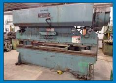
100 Ton X 12' Wisconsin Model 12TM-100 Mechanical Power Press Brake
