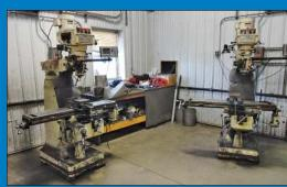
(2) 3-HP Jet Model JTM-4VS Vertical Milling Machines
