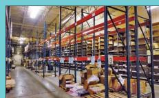
(56) Sections 42" Deep X 144" Wide X 16' High Adjustable Beam Pallet Racking, 3" X 3" Uprights
