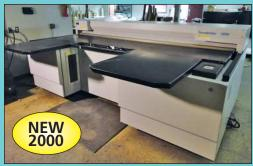
Creo Model Thermoflex 2630S Flexographic Narrow Format CTP Machine
