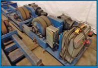
60 Ton IRCO Model 60TON Motorized Tank Turning Roll Set w/ Idler
