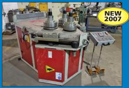
3" x 3" x 5/16" AK Bend Model APK-81 Hydraulic Horizontal Angle, Flat and Tube Bending Roll
