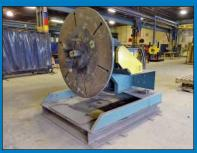
7,500 Lb. Pandjiris Model 75MVRMT Tilting and Rotating Welding Positioner
