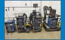
(4) 450 Amp Miller Pipe Pro 450RFC Welders w/ Model Pipe Pro 12RC Suitcase Wire Feeds
