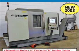
Gildemeister Model CTX-420 Linear CNC Turning Center with Live Tooling, C and Y Axis
