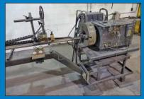
Bug-O Model SEC-1590-E Saddle and Elbow Plasma Pipe Beveling Machine
