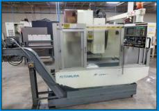
**Kitamura Mycenter-3X CNC Vertical Machining** Center
