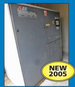
50 HP Atlas Copco Model **GA37FF Self Contained Air Compressor with** Refrigerated Air Dryer
