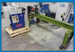
3" LNS Model PB-80 Chamfering Machine & 3" Custom Bar Chamfering Machine with 8" Chuck, 6' **Rail Support**
