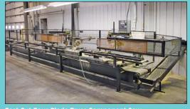
**Fast Cut Four-Blade Truss Component Saw**
