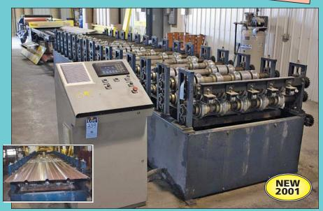
Metal Rollforming Systems 16-Stand Rafted Type Building Panel Rollforming Line
