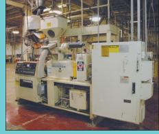
1/8" Cincinnati Milacron Model CM-55 Twin **Screw Extrusion Machine**
