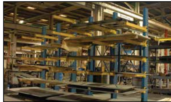
Cantilever Racking w/Partial View of Plate Steel Inventory
