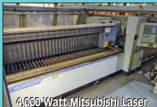
4,000 Watt Mitsubishi Laser
