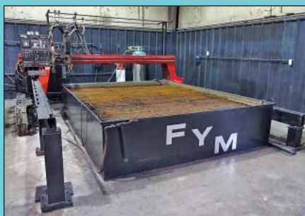
9' X 11' Messer Model Apollo HSG-8 CNC Plasma Table
