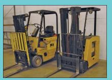
Overall View of Stand Up and Sit Down Electric Lift Trucks
